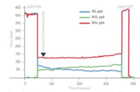
Figure 3 - Trace of NO/NO /NO , concentration during the ISO test for sample PCRETI Coatin
