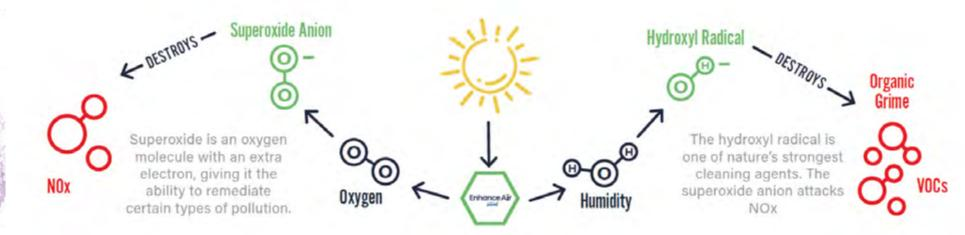
When UVA light energy activates the coating, it starts a chemical process that turns nearby oxygen and water vapor into two powerful cleaning agents ( $OH^{-*}$  and  $O2^{-*}$ )
