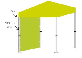
4) From inside the gazebo attach the walls (if ordered). Attach the velcro strip at the top of the wall to the Velcro strip on the indside of the canopy edge. Wrap the Velcro tabs around the gazebo legs.
